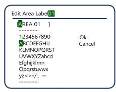
The highlighted portion of the label is the current cursor position, and entering a letter moves the cursor to the right.
