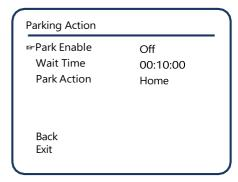
Park Enable: Used to set the activation of the Parking Action function. [On/Off]
