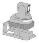
**3)** Insert the camera bracket into the wall bracket's groove as shown in the picture.
