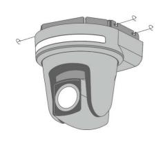
3) Insert the camera bracket into the ceiling bracket's groove as shown in the picture.
